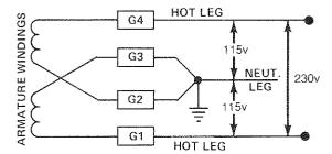
CAUTION: ALL 115 VOLT LOADS MUST BE DIVIDED UP AND CONNECTED IN SUCH A MANNER THAT CURRENT FLOWING IN ANY OF THE THREE LEGS (G1, G4, G2/G3) DOES NOT EXCEED THE LOWEST AMPERAGE RATING ON THE DATA PLATE.
