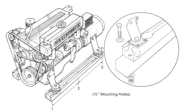
Three 1/2 inch bolt holes are in each generator mounting rail to be used in properly securing the generator to its mounting platform. These holes are on 15 inch mounting centers.
