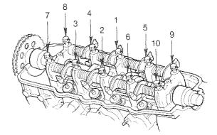
Head bolt tightening torque:
