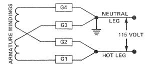
2. WHEN THE ELECTRICAL SYSTEM IS A THREE WIRE TYPE REQUIRING 120V. OR 120/240 VOLTS:
