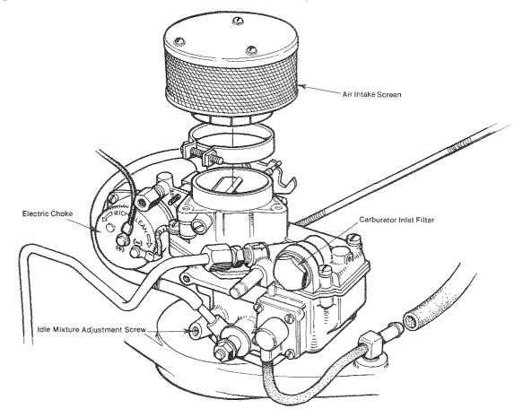
NOTE: Choke index mark is located on the choke cover lower right inboard side.
