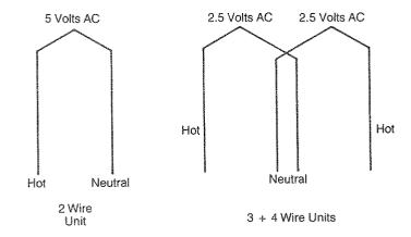
2-wire unit 5 Volts AC (Hot lead to neutral)
