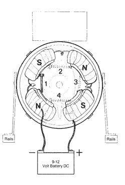
the 9 - 12 volts excitation of the field coils. Should this fail to happen between any of the four adjoining coils/shoes, then an incorrect coil is installed and must be removed and the correct one installed; otherwise the generator when assembled will not produce proper voltage.
