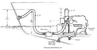
(e) Hydro hush mufflers should be mounted as close to the generator as possible and the exhaust/cooling water mixture from the exhaust injected elbow should drop down into the muffler.
