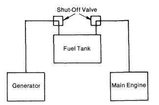
Installations where the generator is located above the fuel tanks should have a shut-off located at the fuel connection to the tank and also a service shut-off valve at the fuel connection to the generator.
